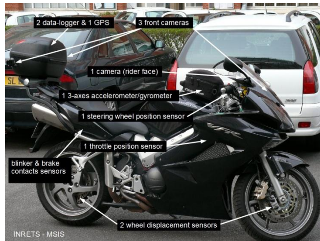
Abbildung 5: Example of instrumented motorbike for pilot naturalistic study
